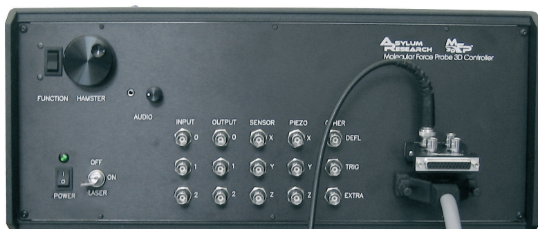
The Digital Access Module easily plugs into the expansion slot in the front of the MFP-3D Controller.
